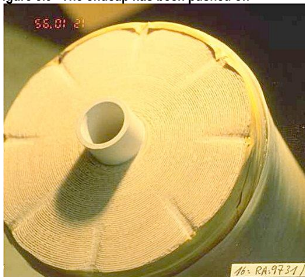
Figure 8.9 The endcap has been pushed off
